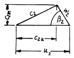
$$\begin{split} Y_{blade} &= U_{2}C_{3U} \ and \ Y_{blade^{\infty}} = U_{2}C_{2u} \\ where, C_{2u} &= U_{2} - W_{2U} = U_{2} - C_{2m} \cot \beta_{2}, \\ Y_{blade^{\infty}} &= U_{2} \left( U_{2} - C_{2m} \cot \beta_{2} \right) and \ it \ follows \\ U_{2} &= \frac{C_{2m}}{2 \tan \beta_{2}} + \sqrt{\left( \frac{C_{2m}}{2 \tan \beta_{2}} \right)^{2} + Y_{blade^{\infty}}} \end{split}$$
