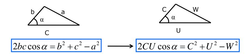
$$Y_{blade} = \frac{1}{2} \left( C_3^2 + U_3^2 - W_3^2 - C_0^2 - U_0^2 + W_0^2 \right)$$
