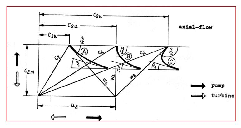
• Three different axial-flow vanes, namely form A, B, C for which  $U_2$ ,  $C_{2m}$  and  $\beta_1$  are the same but the angle  $\beta_2$  differ
